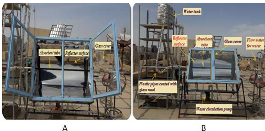
Fig. (4): The trough solar collector parts
