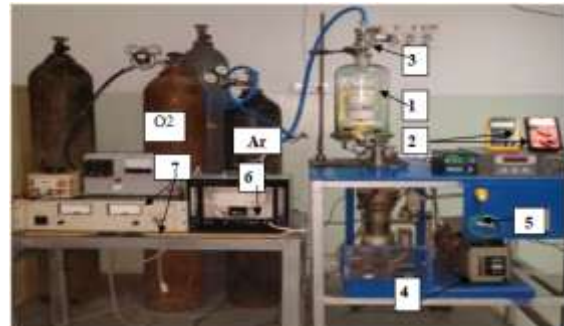
Fig.(2) a photograph of the main experimental set-up used in this work.(1) plasma chamber ((a) cathode (b) anode )) (2) ammeter and voltmeter (3) needle valve(1-160 sccm) (4) vacuum system (5) current limited discharge resistance (6) flow meter and gas mixer (7) H.V power supply
