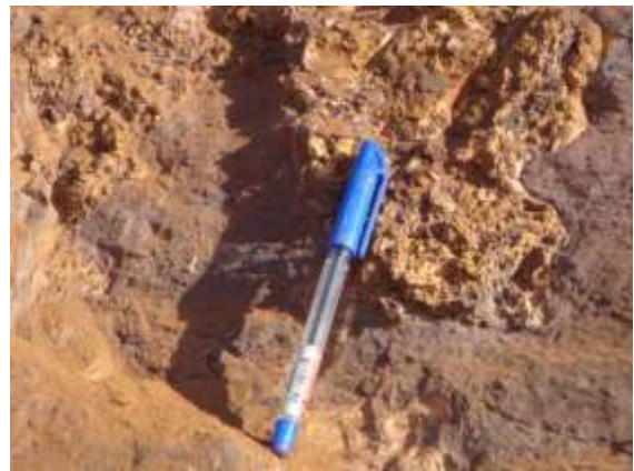
Fig.(6): Visible U-mineralization of sandy siltstone of Adadia Fm. at Ramlet Hemiyr looking S.
