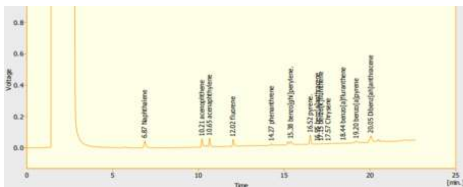
Fig. 3: chromatograms of a standard mixture containing thirteen polycyclic aromatic hydrocarbons at a concentration of 5 ppm.
